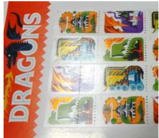
Error pane highlighted to show die cut shift
